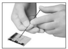
•Keep the cassette flat after the sample has been applied. WARNING: Allowing the sample to sit in the cassette will cause inaccurate results. Immediately place the cassette into the drawer of the analyzer. The black reaction bar must face toward the analyzer. The brown magnetic stripe must be on the right.
