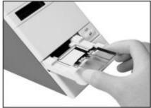
•DO NOT PUSH IN THE DRAWER. Press RUN. The drawer will close. During the test, the screen will display:
